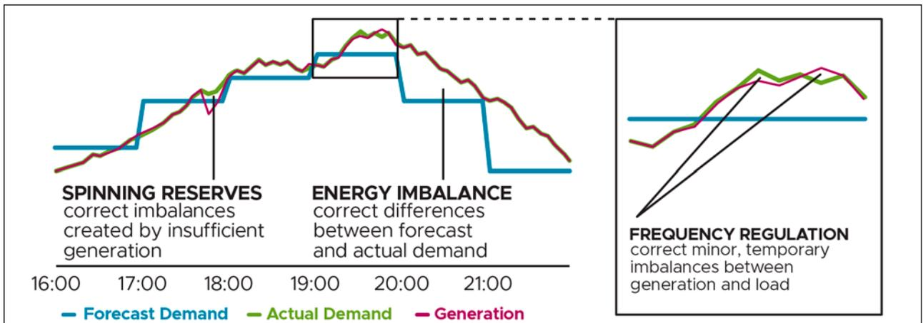
FIGURE 1 Sample illustration of electric ancillary services during peak hours, 4:00–9:00 pm.
