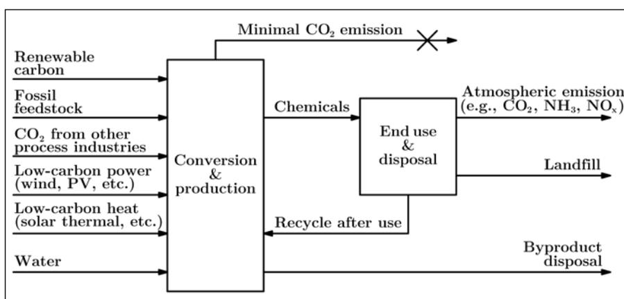
FIGURE 2 A chemical system allowing continued use of significant quantities of fossil resources as feedstock while dramatically reducing greenhouse gas emissions. PV = photovoltaic.
