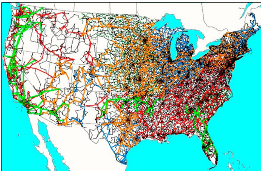
FIGURE 2 Synthetic grid for the contiguous United States. Colors correspond to different nominal transmission line voltages: green = 765 kV, orange = 500 kV, and red = 345 kV. Source: Texas A&M University Electric Grid Test Case Repository ([electricgrids.engr.tamu.edu](http://electricgrids.engr.tamu.edu)).
