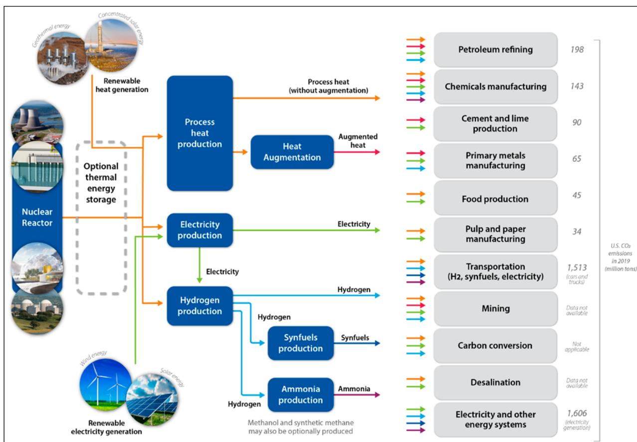
FIGURE 1 Illustration of possible energy generation and use options for an integrated energy park, showing energy flows and input requirements for energy users. Adapted from Foss et al. (2021).
