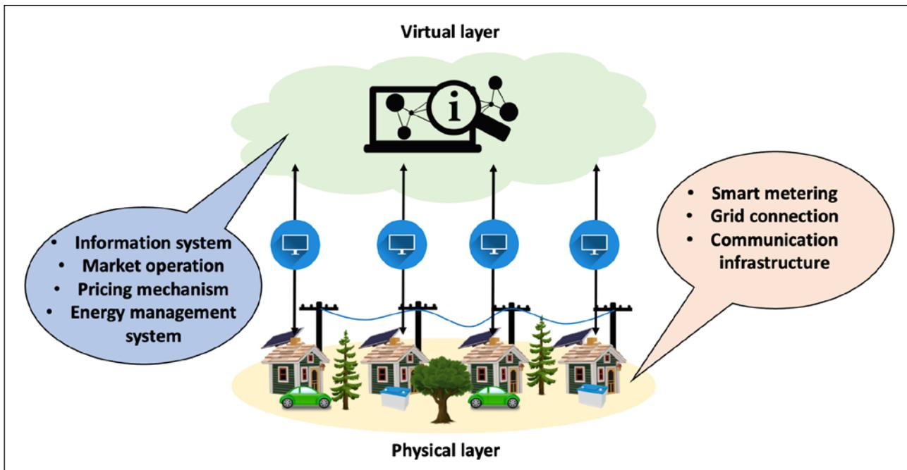
FIGURE 1 The virtual and physical layers of a peer-to-peer network and their elements. Adapted from Tushar et al. (2021a), where the details of different elements are also explained. Images are royalty-free and taken from <https://pixabay.com/>.
