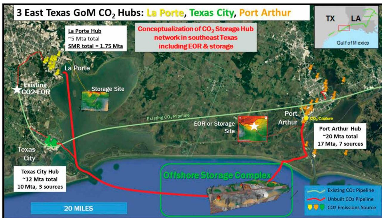
FIGURE 1 Conceptual diagram of potential carbon capture and storage hubs in Southeast Texas. EOR = enhanced oil recovery; GoM = Gulf of Mexico; Mta = megatons per year; SMR = steam methane reforming. Reprinted with permission from Meckel et al. (2021).
