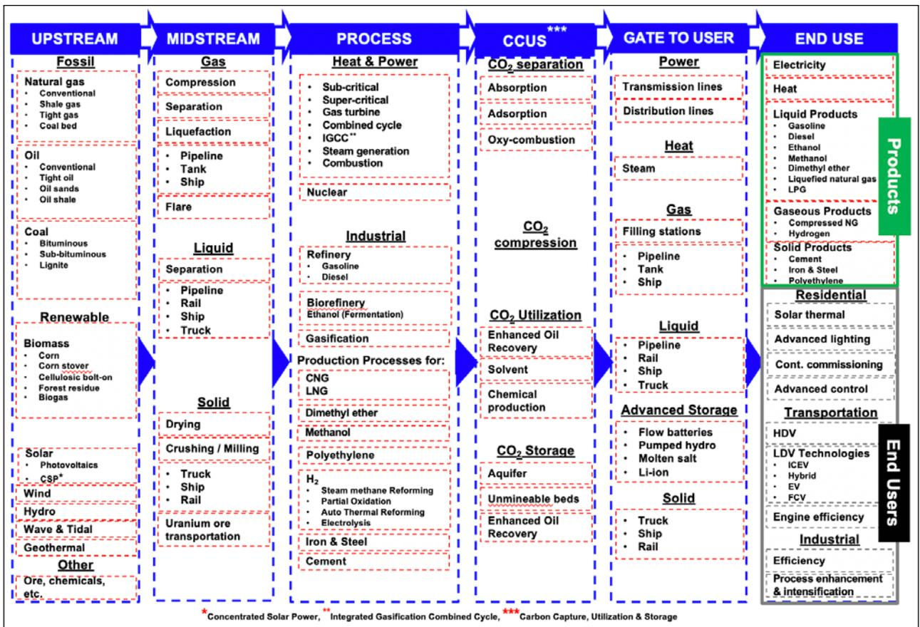
FIGURE 2 The MIT Sustainable Energy System Analysis Modeling Environment (SESAME) has a modular structure with six lifecycle stages. Existing and new energy pathways can be constructed and analyzed for lifecycle emissions and cost by combining modules in the six columns. Reprinted with permission from Gençer et al. (2020).
