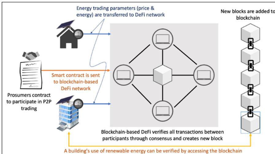
FIGURE 2 How a blockchain-based decentralized finance (DeFi) network can help houses and buildings track their 24/7 use of renewable energy in peer-to-peer (P2P) trading and reduce carbon taxes. Images used in the figure are royalty-free and taken from <https://pixabay.com/>.
