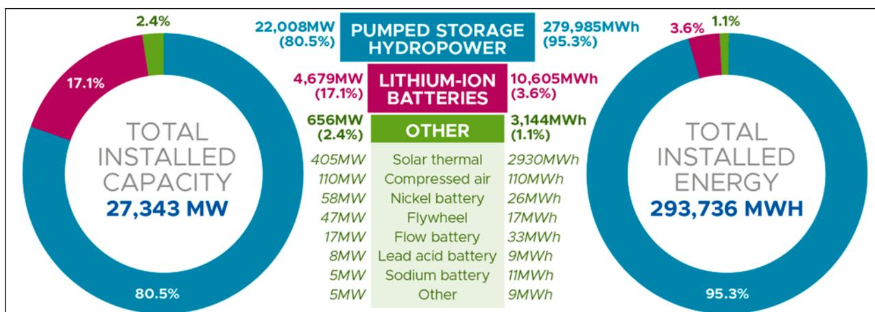
FIGURE 2 Installed energy storage capacity (left) and output (right) by technology in the United States, 2021 (data from EIA 2023). MW = megawatts; MWh = megawatt-hours.
